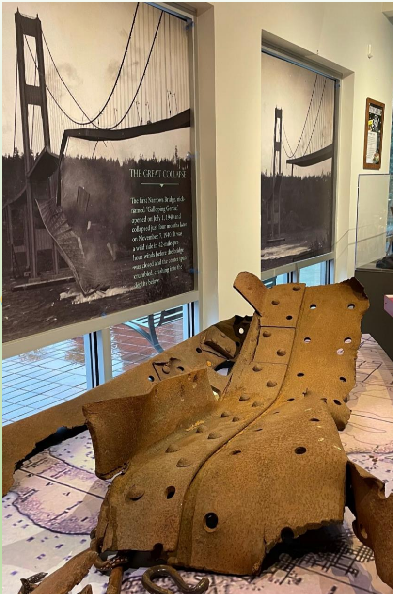
Pieces of steel believed to be from Galloping Gertie. Found underwater while building the 2007 Narrows Bridge. On display at Harbor History Museum. Donated to HHM by the Washington State Department of Transportation, which operates and maintains the bridges today.
